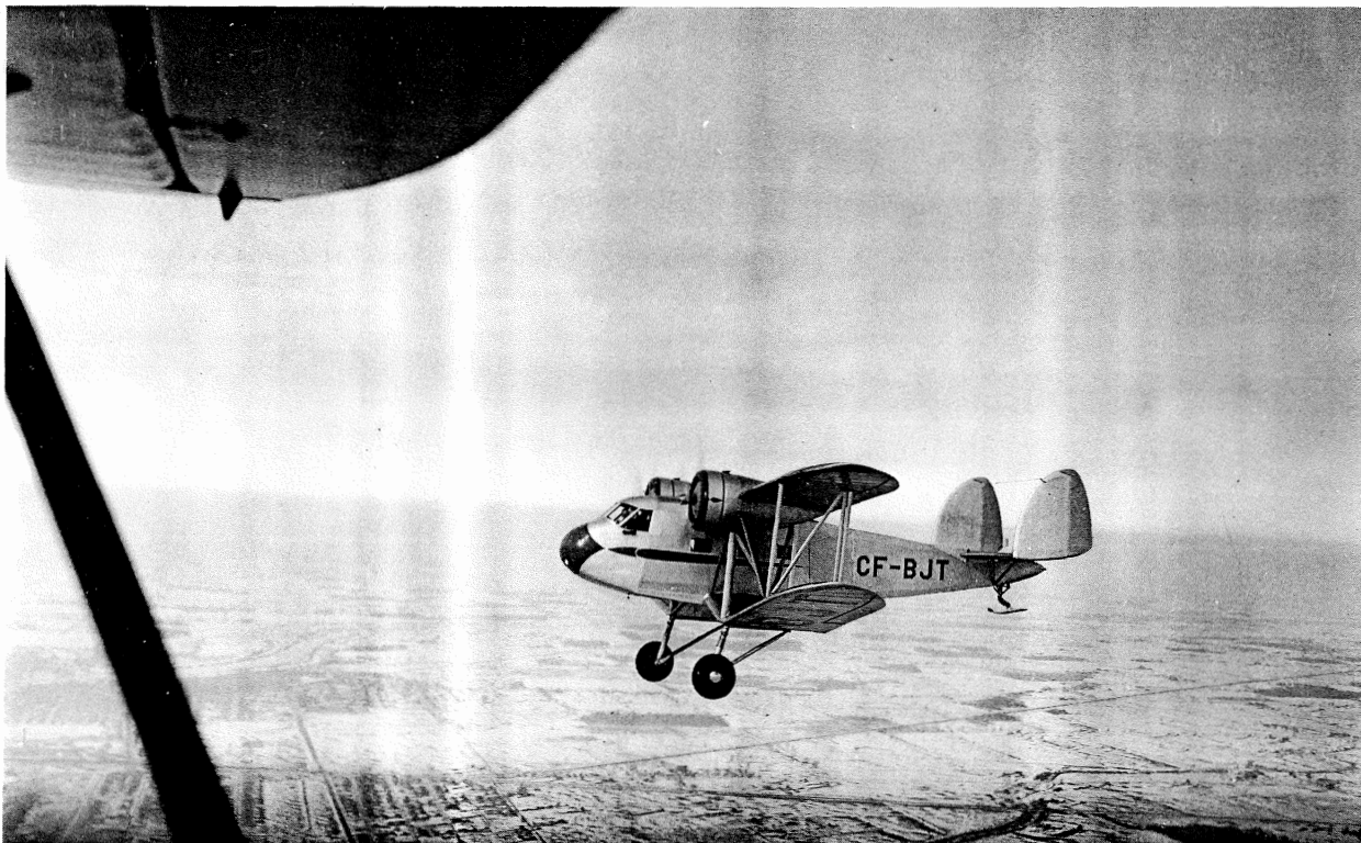
A rare view of the passenger version of the Fleet Model 50K CF-BJT airborne. Note the tailskid instead of a tail-wheel. – B. MacRitchie Collection
