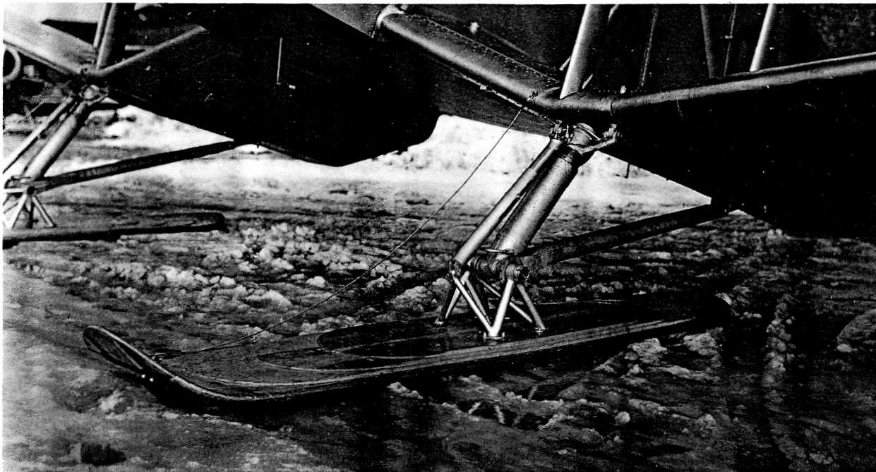
A close-up of the ski installation on the Fleet Freighter. – B. MacRitchie Collection
